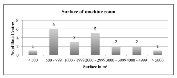
The variety of machine room size within the sample is shown in Figure 4 below:
