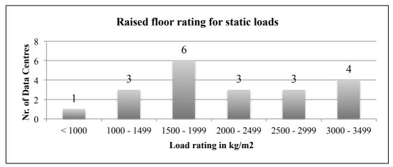
Figure 8: Raised floor rating for static loads  $(kg/m^2)$
