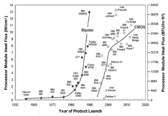
Figure 2: Evolution of processor module level heat flux in high-end servers. ASHRAE 2016, p. 27
