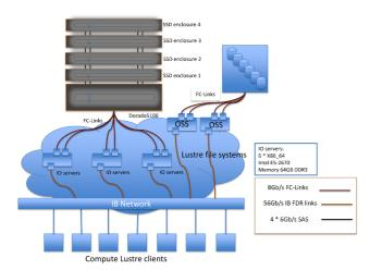
Figure 5. Schematic showing the test environment used for the Lustre testing including IO servers, Dorado5100 as metadata storage, some additional data storage and compute clients.
