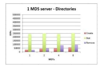
Figure 7. mdtest results for directory operations using a single metadata server (MDS) with 1 to 8 metadata targets (MDTs).
