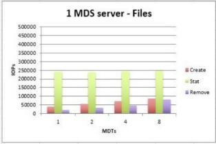
Figure 8. mdtest results for file operations using a single metadata server (MDS) with 1 to 8 metadata targets (MDTs).
