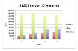
Figure 9. mdtest results for directory operations using a 2 metadata servers (MDSs) having from 2 to 16 metadata targets (MDTs).
