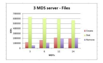
Figure 12. mdtest results for file operations using a 3 metadata servers (MDSs) having from 3 to 24 metadata targets (MDTs), i.e. 1 to 6 director blades.
