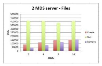
Figure 10. mdtest results for files operations using a 2 metadata servers (MDSs) having from 2 to 16 metadata targets (MDTs).
