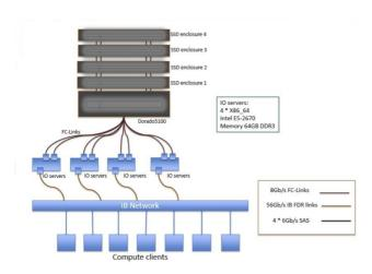
Figure 3. Schematic showing the test environment used for the FIO testing including storage, IO servers and compute clients.
