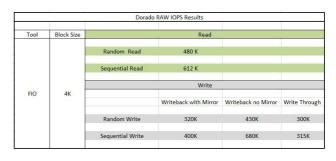
Figure 4. FIO IOPs results running on 4 servers - 128 threads (32 threads per server).
